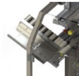
Semi-automatic product feeding unit.
